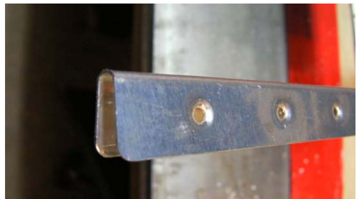
Finished Aileron rib.
