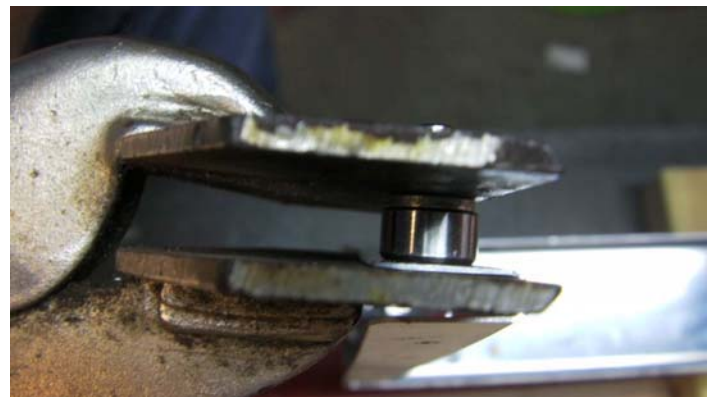
Dimple die installed.
