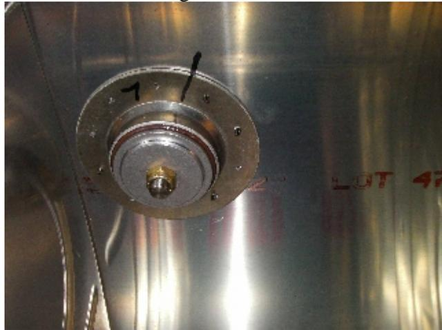
Now I am ready to put in the tank baffle, so all the holes in the fuel tank ribs can be drilled to the correct size. After Drilling the holes, I set up the countersink for the holes at the tank baffle location, and countersunk all the holes. Testing them with a rivet.
