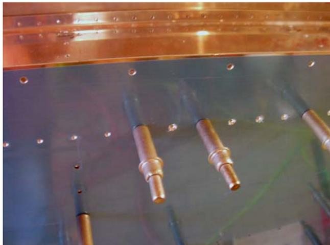
Well, the only thing left at this point is to countersink the tank mounting holes and dimpling, which I will wait To get some help. So I put the tank back onto the spar and drilled the holes where the tank meets the leading Edge.
