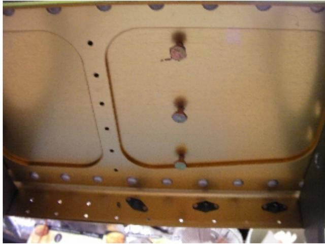
More parts are need for the fuel tank, I made the stiffeners as per the dwg. and clecoed them into place.
