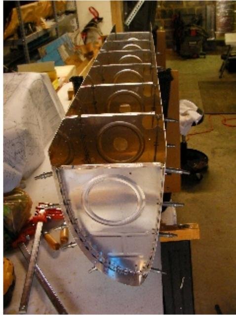
Time to work on the fuel tank baffle, used the template to locate the hole in the middle of each Z bracket. Clecoed them to the baffle, squared each bracket and drilled all the holes. Put the baffle on the main spar, and located the mounting holes for the Z brackets. Drilled the mounting holes, and then used a platenut jig to drill the rivet holes, and then countersunk those holes.
