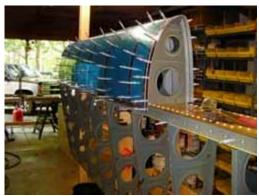
I decided to work on the fuel tank baffle and z brackets next, so I used the drill jig provided to locate the first hole in each
