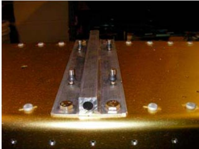
Wing hold down piece installed after fabrication.
