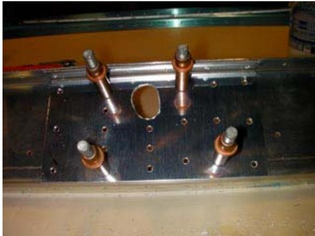
A doubler plate on the lower spar after drilling, in place after cutting the aileron tube hole to match the spar.
