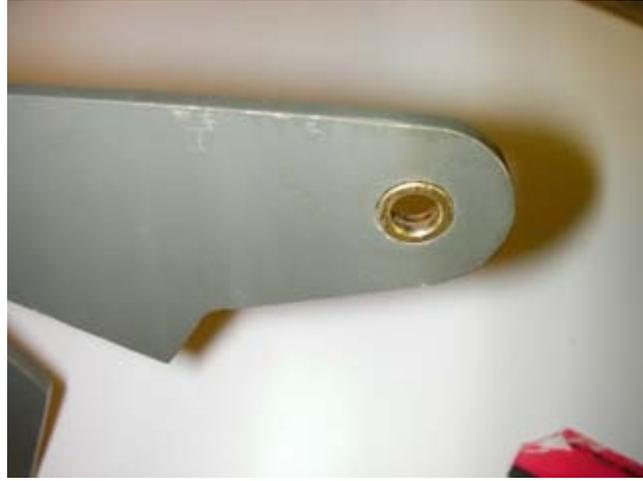
**All the lower ribs clecoed into place, also the aileron brackets, and flap brackets with reinforcing angles, they are made By cutting miters, and drilling in place. After drilling, more deburring.**
