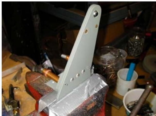
**I used a bolt and nut to hold the bearing for the flap bracket for sanding to the right**
