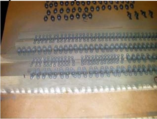
**Riveted the platenuts to the main spar.**
